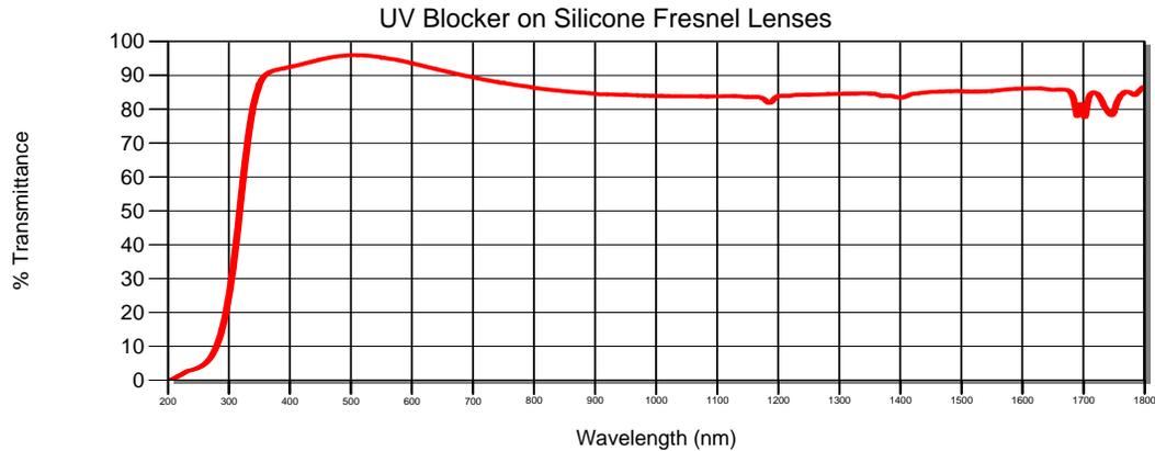
Figure 3: Measured spectrum of silicone (DC93-500) Fresnel lens, providing UV blocking and high transmission
